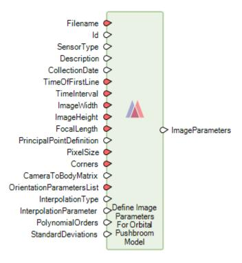
This defines the parameters which describe an image collected using an orbital pushbroom sensor. Additionally, parameters related to how the sensor is modelled or adjusted for the particular image may be specified in the InterpolationType, InterpolationParameter, PolynomialOrders and StandardDeviations options.
