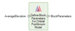
This defines the parameters needed to create a block for the management of orbital pushbroom images.
